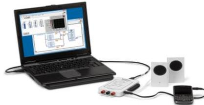
Analog output allows us to send a continuous signal that varies within a specified range from our data acquisition card to a sensor or another application if applicable. In our case we are sending our modified audio signal to the speakers or headphones so we can hear the changes that our filter is implementing.
