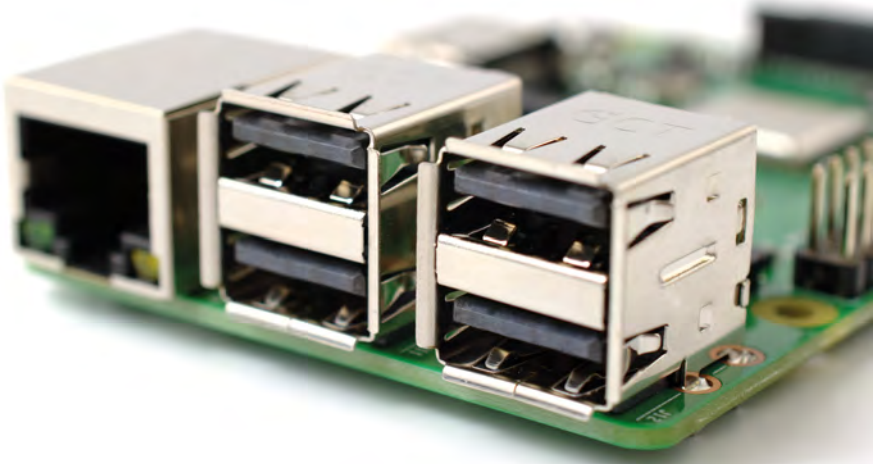
▲ Figure 1-6: The Raspberry Pi's USB ports
