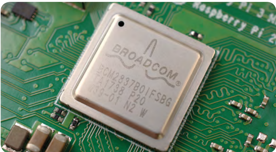
◀ Figure 1-2: The Raspberry Pi's system-on-chip (SoC)
