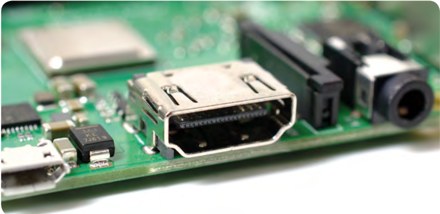
▲ Figure 1-10: The Raspberry Pi's HDMI port
