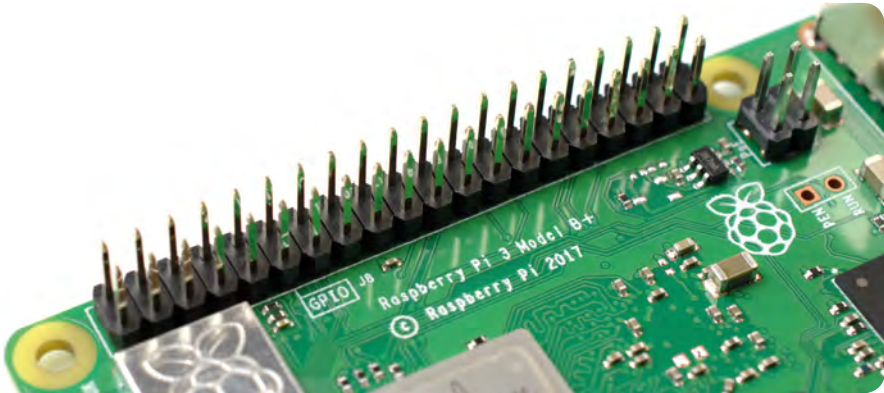
▲ Figure 1-14: The Raspberry Pi's GPIO header
