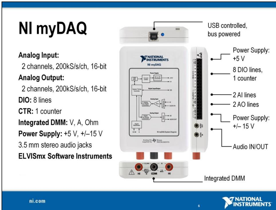
NI myDAQ is a low-cost portable data acquisition (DAQ) device that uses NI LabVIEW-based software instruments, allowing students to measure and analyze real-world signals. NI myDAQ is ideal for exploring electronics and taking sensor measurements. Combined with NI LabVIEW on the PC, students can analyze and process acquired signals and control simple processes anytime, anywhere.
